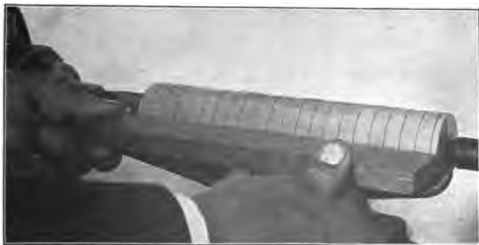
Fig. 36. Using a Gauge Stick.
